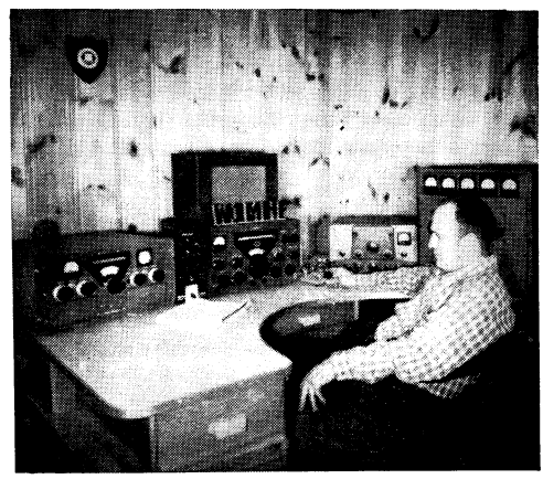
During SS this neat and spacious station was crammed with a Viking I, Ranger, and HT-32, and three separate bugs with all rigs on different bands . . . instantaneous bandswitching you know. Slouching down in the operating position is W1MHF, who led Connecticut with 180,000.
