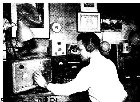
With this spiffy layout, John Ryan, W7KVU, brought home a blistering 202,210 points and the Montana wall-paper. When he feels like creating additional db. for DX chasing, John uses the B & W 5100 to excite p.p. 4-400As at one kw.
