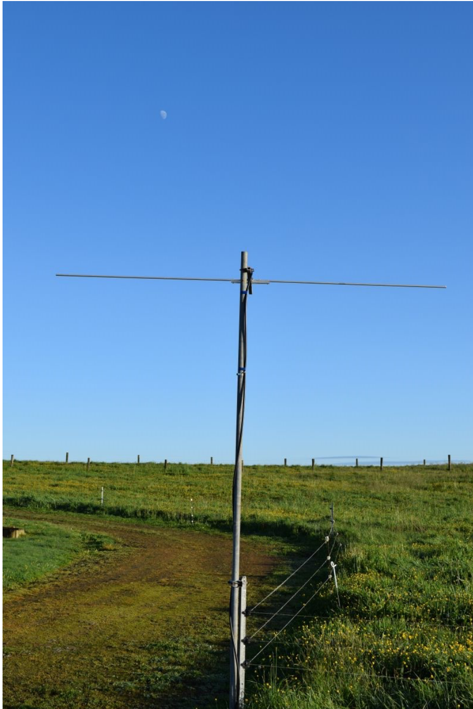
1-element 'yagi' by ZL1RS
