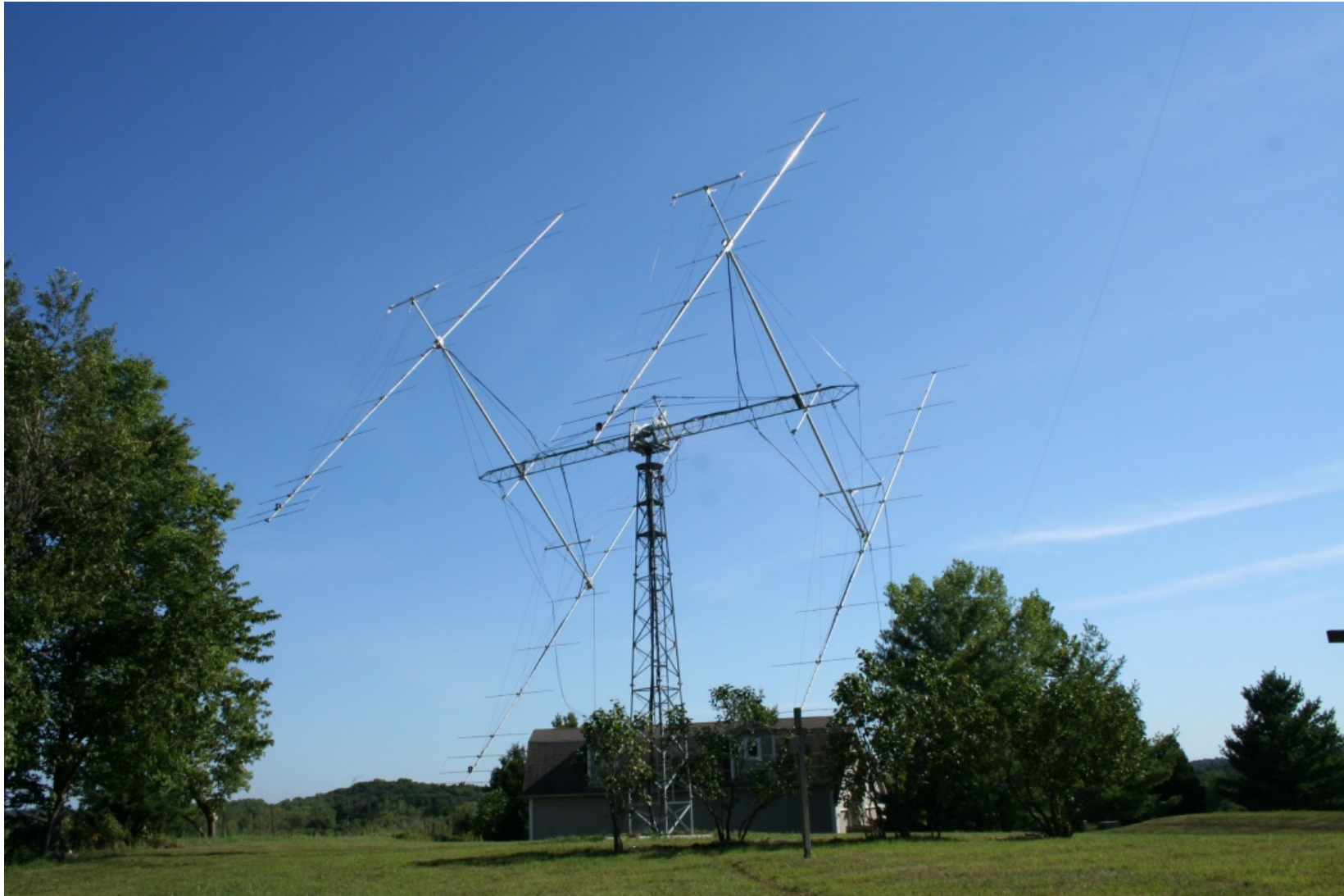
KJ9I 6m EME array: 4 x 10-LFAs rotated by Extra-Large prop-pitch (azimuth) and Small prop-pitch (elevation). Photo by KJ9I
